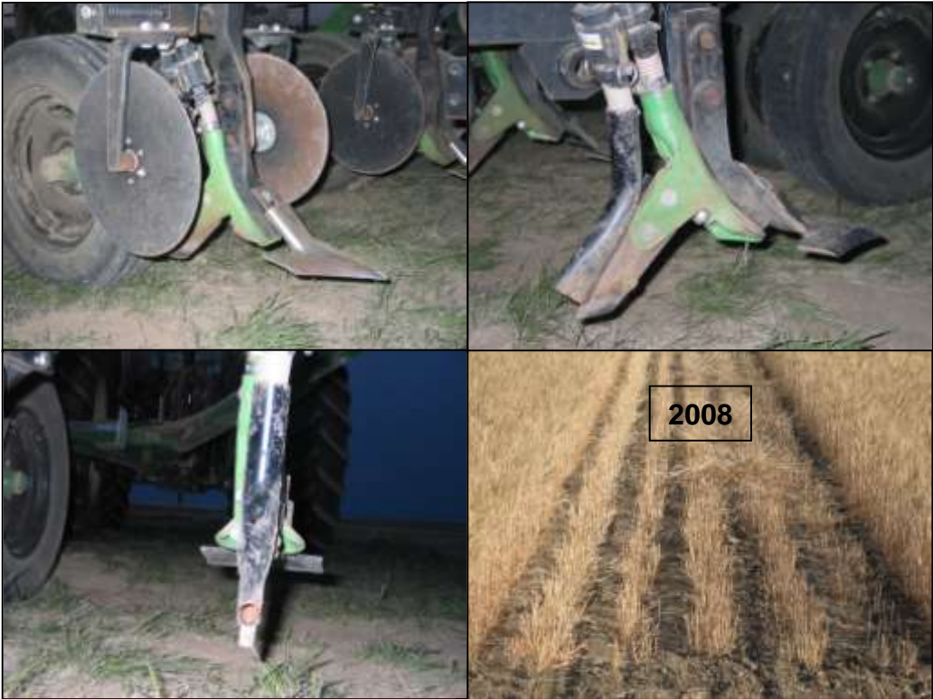
Figure 4. FARMLAND SB1-SBS1 w/ 6" Sweep & Backswept Knife (Solid, Seed Band Width = 5.8 Inches)
