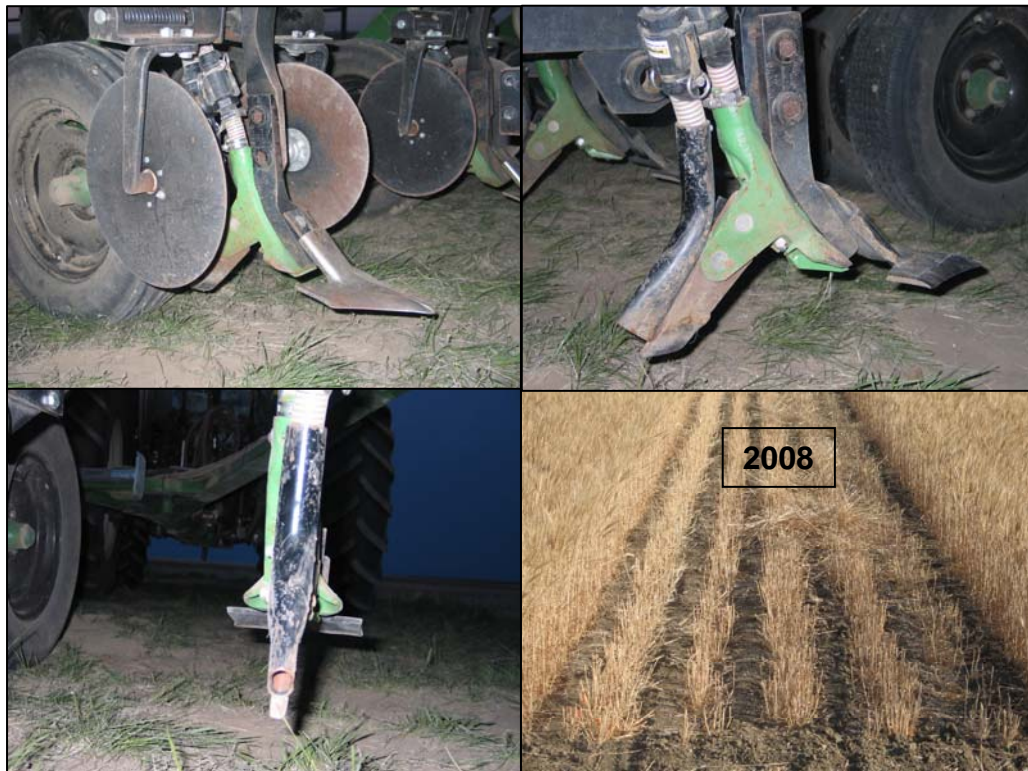
Figure 5. GEN 200 T2x2 Paired Row (Row Style = Paired/Separate, Seed Band Width = 6.9 Inches)
