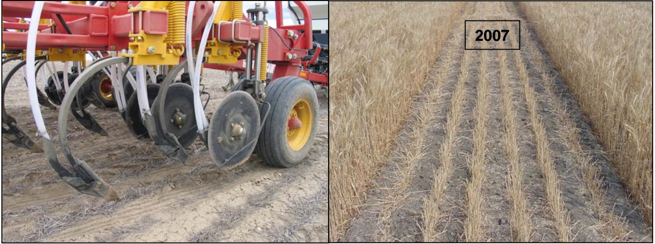
Figure 9. BOURGAULT Sngl-Shoot: 20-40-0 w/Seed+50-0-0 via PP-Bd'Cst (Solid, Seed Band Width = 3.3 Inches)
