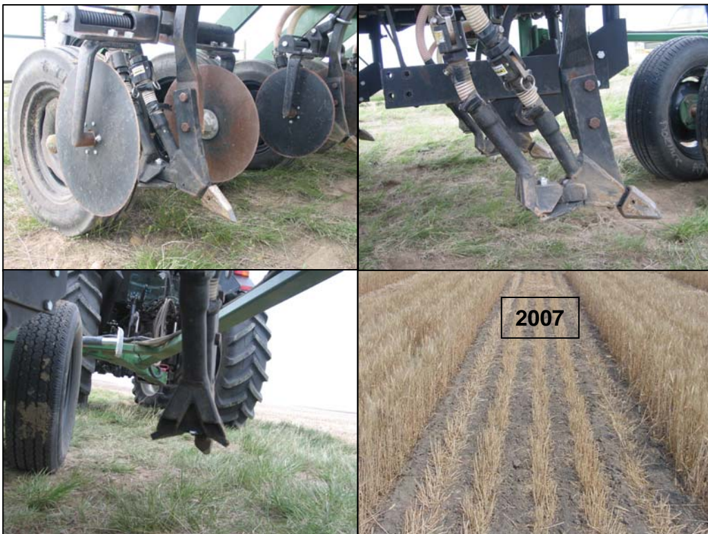
Figure 2. DUTCH 3.5" Paired Row (Row Style = Solid, Seed Band Width = 5.4 Inches)
