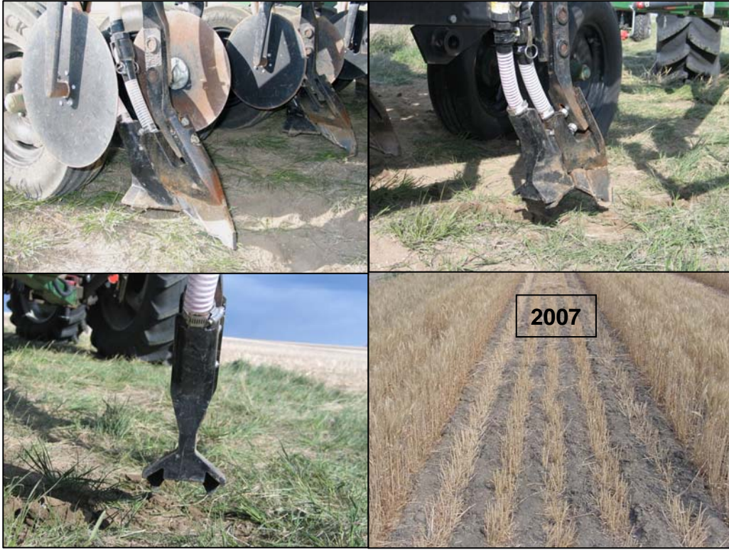
Figure 1. BOURGAULT 3" Paired Row (Row Style = Solid, Seed Band Width = 5.4 Inches)
