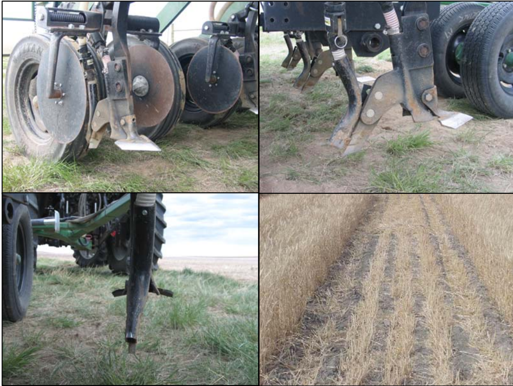
Figure 7. FARMLAND LD w/ 6" LD Sweep & Backswept Knife (Solid, Seed Band Width = 5.3 Inches)
