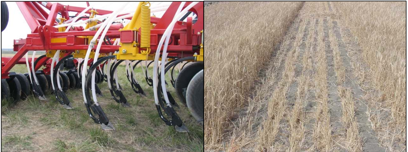
Figure 20. DUTCH Low Draft Dbl-Shoot: 8.5-40-0 w/Sd+61.5-0-0 via FertBnd (Paired/Joined, Band Width = 5.4 Inches)
