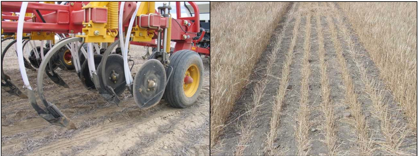
Figure 14. BOURGAULT Single-Shoot: 8.5-40-0 w/Seed+61.5-0-0 via MRBs (Solid, Seed Band Width = 2.7 Inches)
