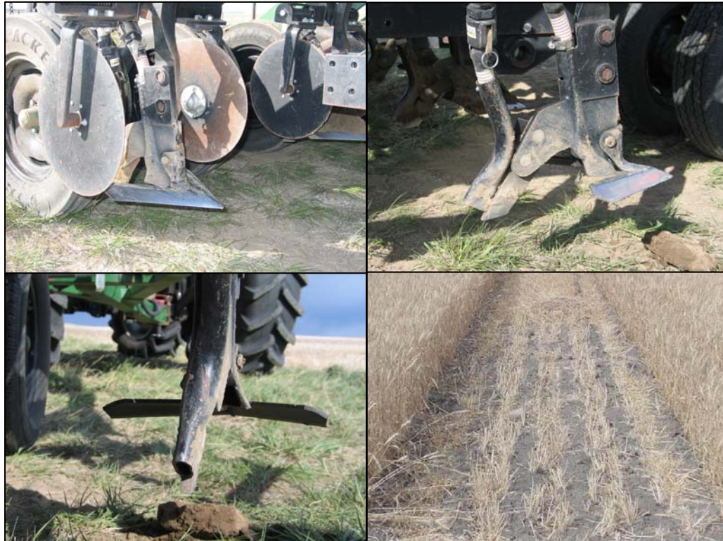
Figure 8. FARMLAND LD w/ 11" LD Sweep & Backswept Knife (Solid, Seed Band Width = 5.9 Inches)
