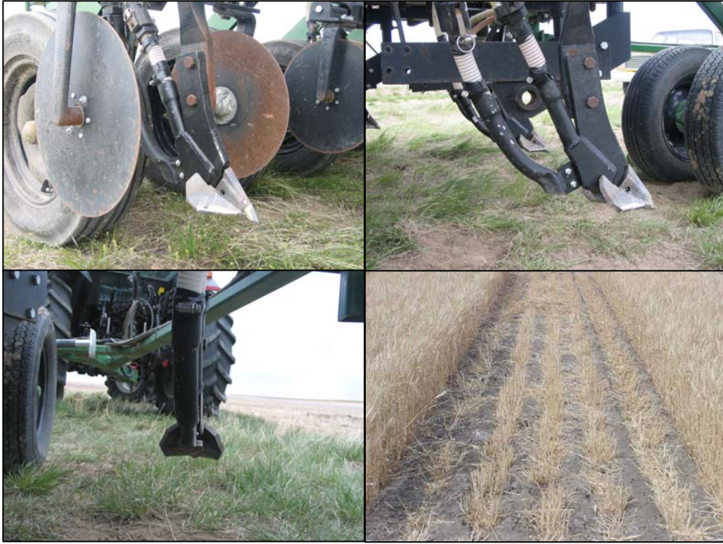
Figure 5. DUTCH Low Draft Paired Row (Solid, Seed Band Width = 5.9 Inches)
