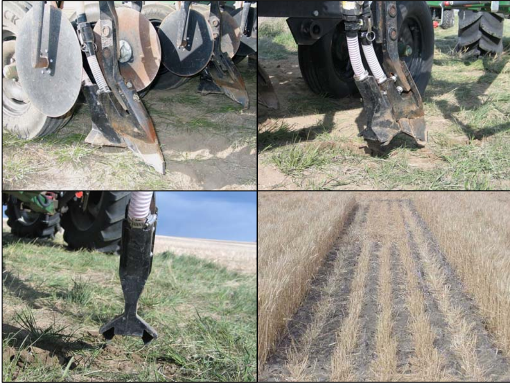
Figure 3. BOURGAULT 3" Paired Row Prototype (Solid, Seed Band Width = 4.8 Inches)
