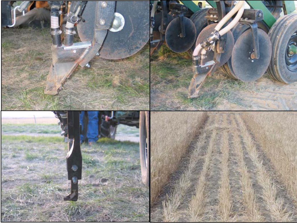
Figure 1. ATOM JET Side Band (Solid, Seed Band Width = 3.4 Inches)
