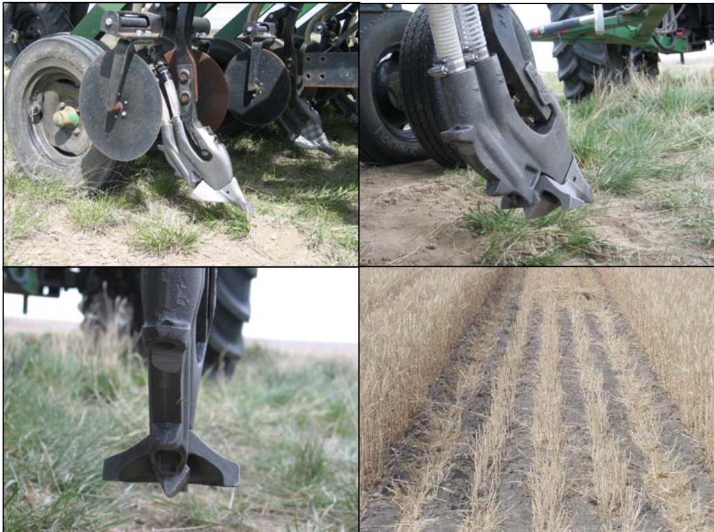
Figure 12. GEN 300 T2 Paired Row (Solid, Seed Band Width = 5.1 Inches)
