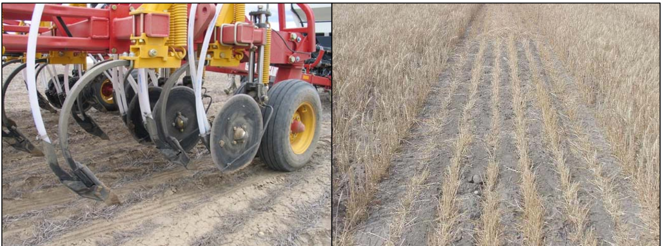
Figure 16. BOURGAULT Sngl-Shoot: 30-40-0 w/Seed+40-0-0 via PP-Bd'Cst (Solid, Seed Band Width = 3.2 Inches)
