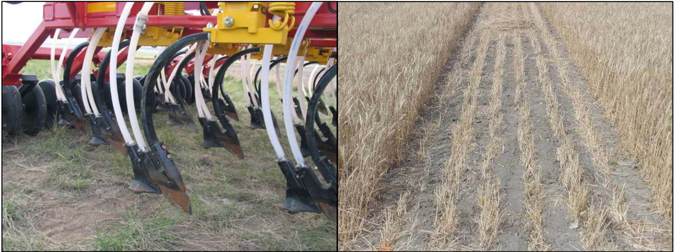
Figure 18. BOURGAULT Dbl-Shoot: 8.5-40-0 w/Seed+61.5-0-0 via FertBand (Solid, Seed Band Width = 5.0 Inches)
