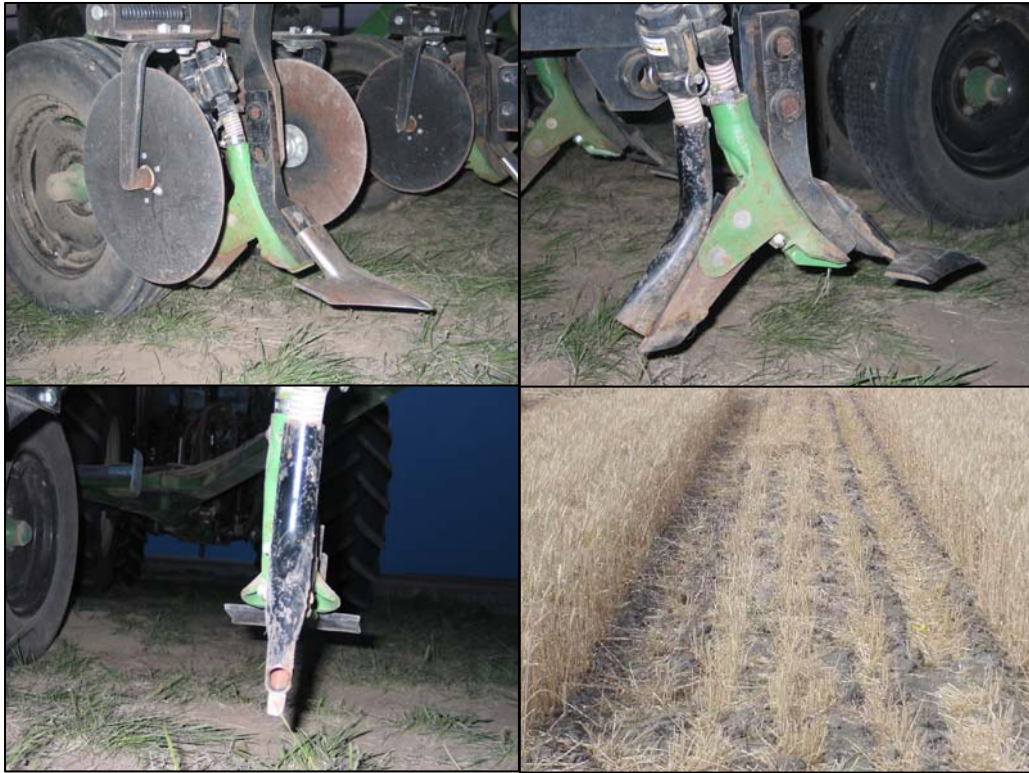
Figure 9. FARMLAND SB1-SBS1 w/ 6" Sweep & Backswept Knife (Solid, Seed Band Width = 5.7 Inches)
