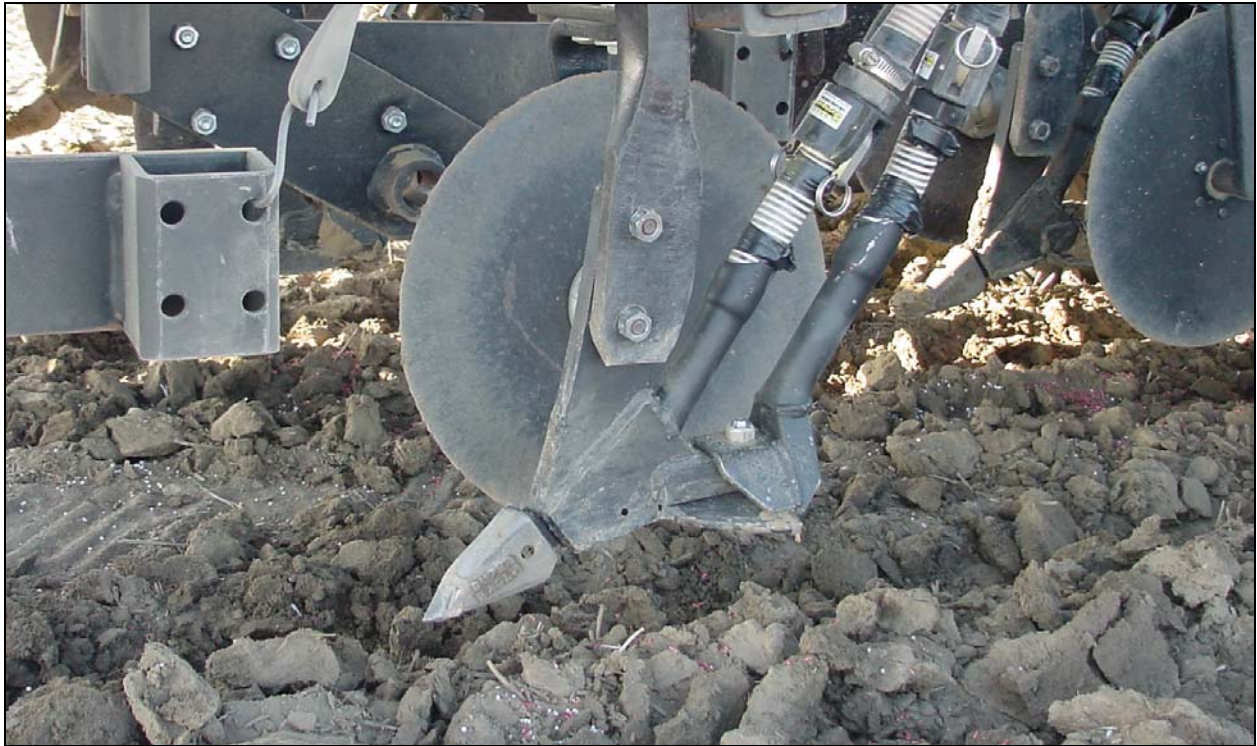
Figure 5a. DUTCH 3.5" Paired Row w/SUPER EAGLE Tip
