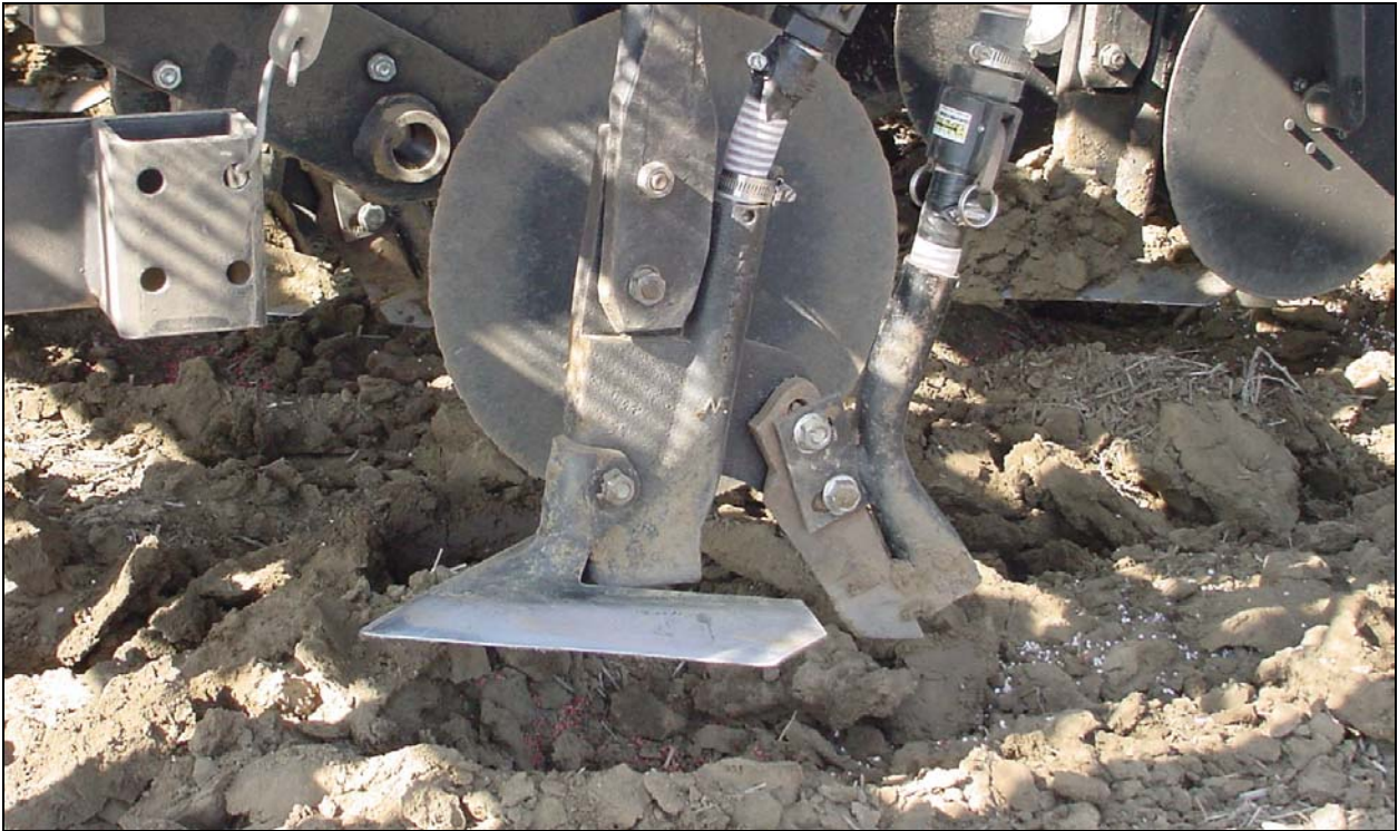
Figure 8a. FARMLAND LOW DISTURBANCE (LD) w/Case-McKay 11" LD Sweep & K3 Backswept Knife
