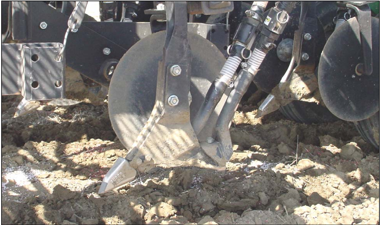
Figure 3a. DUTCH SUPER EAGLE w/3.5" Paired Row Attachment
