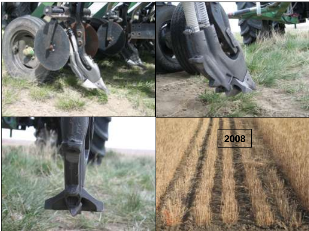
Figure 6. GEN 300 T2 Paired Row (Row Style = Paired/Joined, Seed Band Width = 5.9 Inches)
