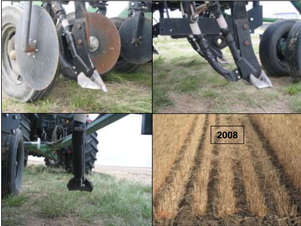
Figure 3. DUTCH Low Draft Paired Row (Row Style = Paired/Joined, Seed Band Width = 6.0 Inches)
